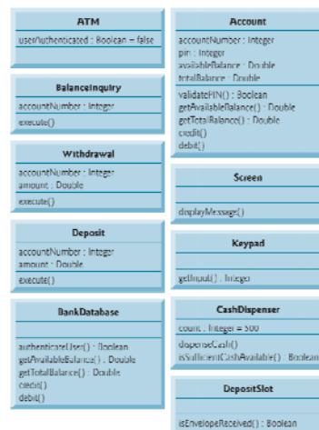
Fig. 12.17 | Classes in the ATM system with attributes and operations.
