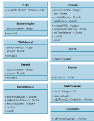
Fig. 13.1 | Class diagram with visibility markers.
