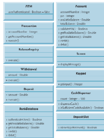
Fig. 13.10 | Class diagram with attributes and operations (incorporating inheritance). Note that the abstract class name Transaction and the abstract
