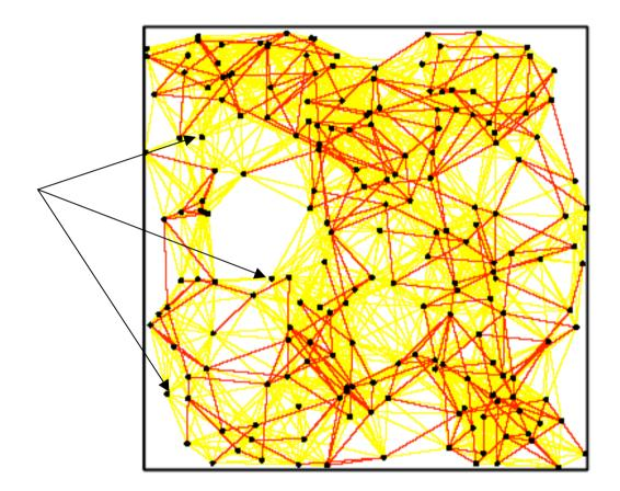
Randomly generated secure sensor network of size 200. Communication range is 0.2, key ring size is 4, and pool size is 100. Lighter lines mean physical visibility, darker lines secure visibility. The network has a few isolated sensors.
