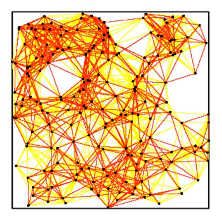
Randomly generated secure sensor network of size 200. Communication range is 0.2, key ring size is 4, and pool size is 50. Lighter lines mean physical visibility, darker lines secure visibility. This graph is connected by using secure links alone.
