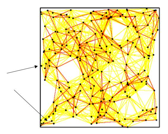
Randomly generated secure sensor network of size 200. Communication range is 0.2, key ring size is 4, and pool size is 150. Lighter lines mean physical visibility, darker lines secure visibility. The network has a slightly larger number of isolated sensors and even some very small disconnected components.
